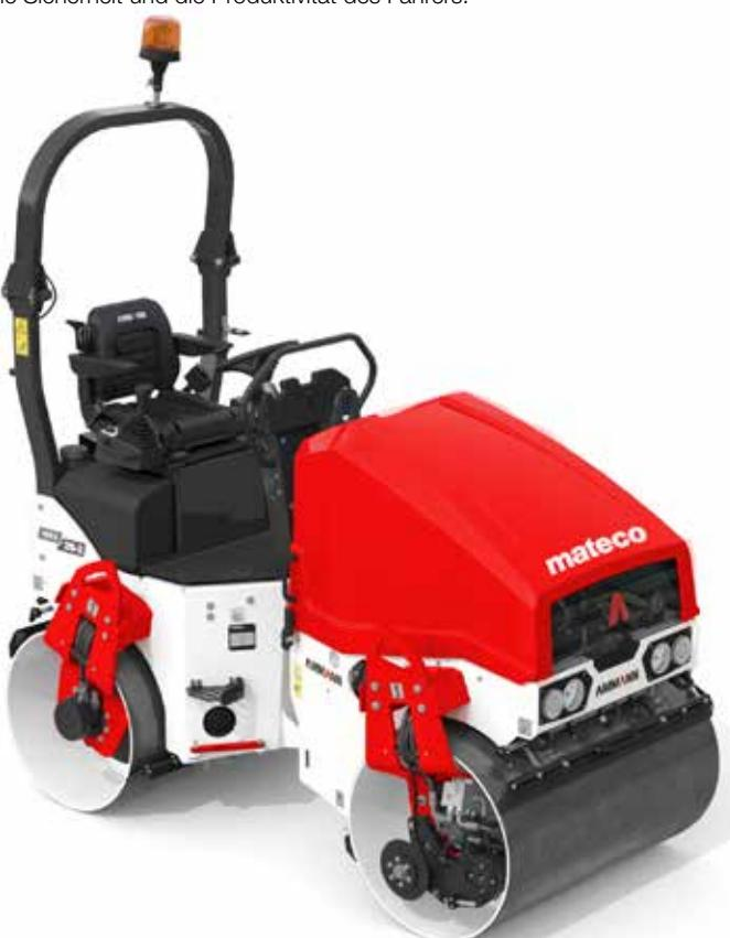
max. Vibrationsfrequenz **66 Hz**
